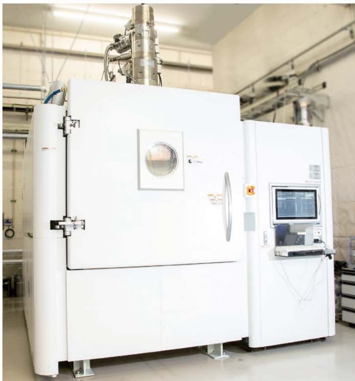
"Prototype Electron Beam Metal AM Machine supported – a TRAFAM project"
